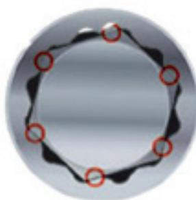
A Snap-on® Flank Drive® wrench moves the contact away from the corners with a radius, then provides flat-to-flat contact for up to 20% more turning power.
