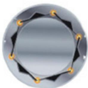
Conventional 12-point wrench and the contact it makes on the corner of a nut or bolt. The corner can round off under high loads causing the wrench to slip.
