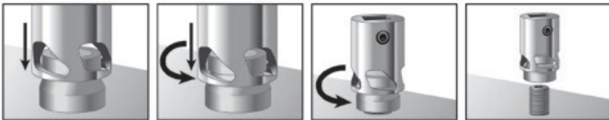
Recently, ATI developed a Hi-Lok® removal socket that has internal teeth that bite into the collar material. Using a Hi-Lok® ratchet or Hi-Lok® Roller Clutch Wrench, the operator places the socket over the collar and turns the ratchet. The socket's teeth dig into the collar material with sufficient force to gain a hold of the collar so that it can be unscrewed. Again, a hex wrench may be used to stop the pin from rotating as needed.
