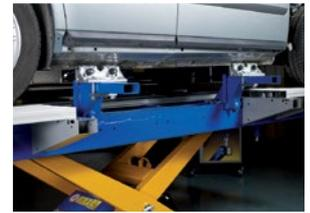
**Secure clamping —** the best grip — no clamping slip. Q63 adjustable bench mountings allow pull while the vehicle is supported on its wheels.
