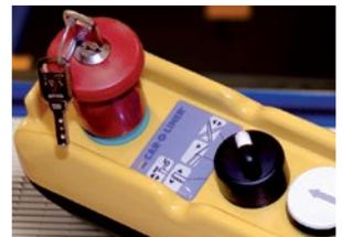
**User-friendly control —** with all-in-one functions for automatic bench tilting, lifting, 10-ton pulling and hydraulic jacking
