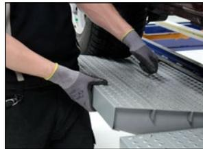
**Removable ramp sections** lift out easily to allow better access to the vehicle
