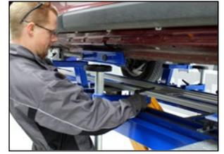
**Exclusive pillar jacks and sill (rocker) supports** make mounting of vehicles fast, safe and easy
