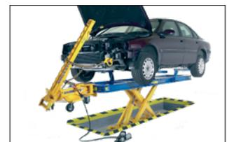
**In-ground installation** — frame is level with floor for easy drive-over
